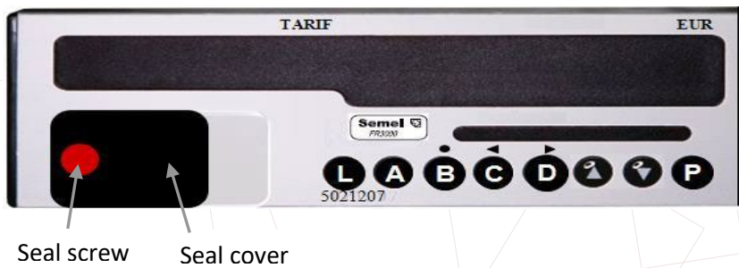
Figure 7: Sealing of displays TD330 i.e. sealing button to allow change of software and flag settings.
